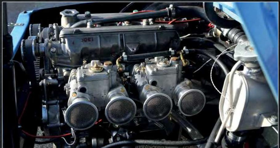
decided to build a 1300 unit based on the Fiat/Lancia 1300, as used in home-market Fiats and Lancia Deltas. This is a super engine with the same crank journal sizes as a 2.0-litre unit and produces around 80hp on a single carburettor. It's a really robust power unit whose bore and stroke of 86.4mmx55.5mm are extraordinarily close to Abarth's 86mmx55mm.
